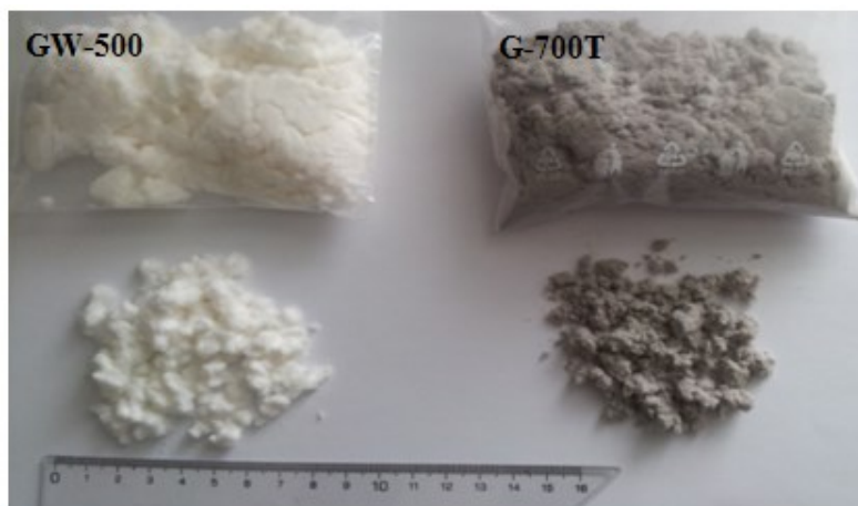
Fig. 1 White (wood pulp) and grey (recycled paper) Greencel cellulose fibres
