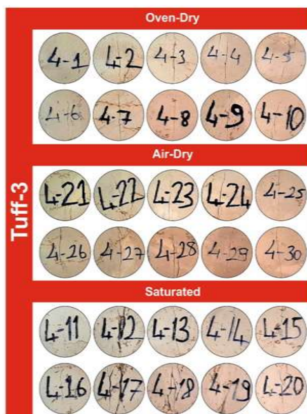
Figure 5. Failure photos of the tuff-3 samples in the Brazilian (indirect) tension tests
