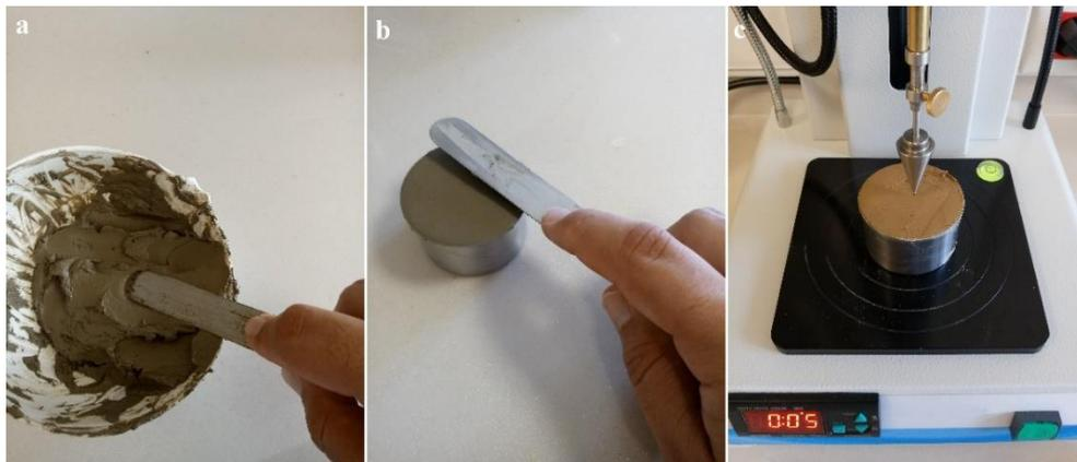
**Figure 2.** a) Soil mixing, b) placing specimen in the mold and surface flattening, c) a prepared specimen under the cone penetrometer
