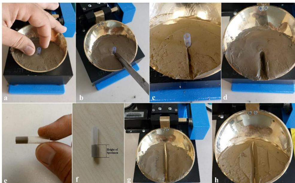
**Figure 3.** a) Tube insertion into the Casagrande test specimen, b) and c) cutting the way to remove the tube, d) a specimen after removing the tube, e) and f) void ratio specimens in the glass tube, g) the groove cut, h) closure of the groove of a tested specimen
