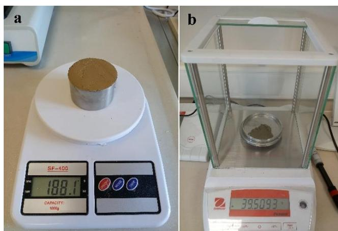
**Figure 4.** Scales used in this study: a) scale with the sensitivity of 0.1 g, b) scale with the sensitivity of 0.0001 g
