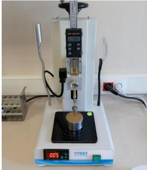
*Figure 1. The cone penetrometer*
