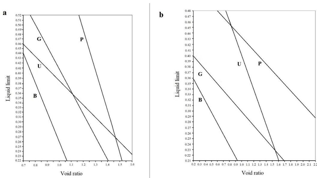
**Figure 5.** Relation between void ratio and liquid limit values obtained from the Cone Penetrometer (a) and the Casagrande test (b)
