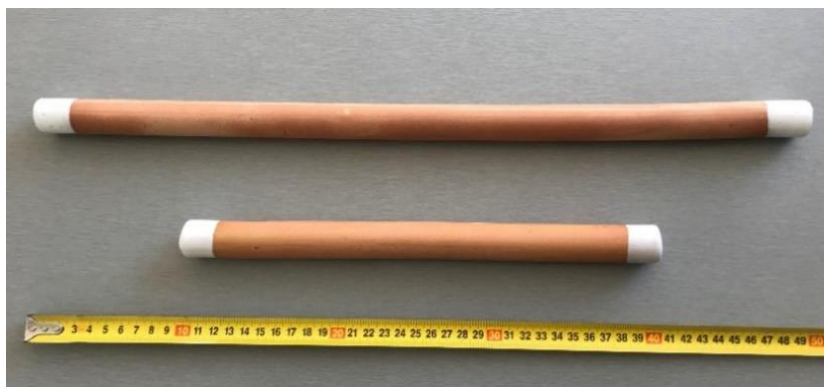
Figure 2. Final support sintered at 1000 °C
