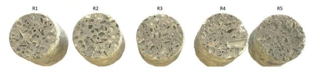
Figure 2. Structure of the test specimens prepared according to formulas R1 to R5
