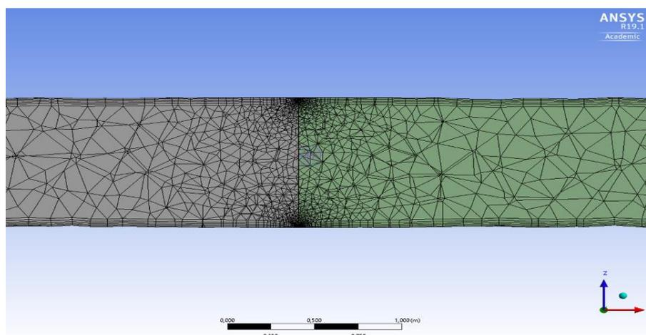
**Figure 3.** *Densification of the computing network in the vicinity of perforation – cross-section*
