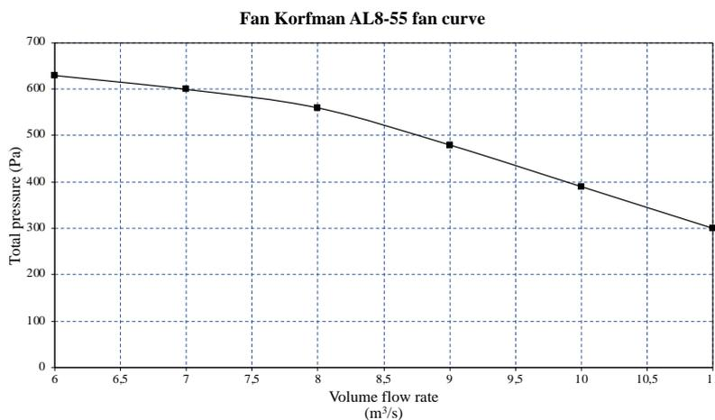
**Figure 2.** Curve of the operation characteristic of Korfman AL8-55 fan
