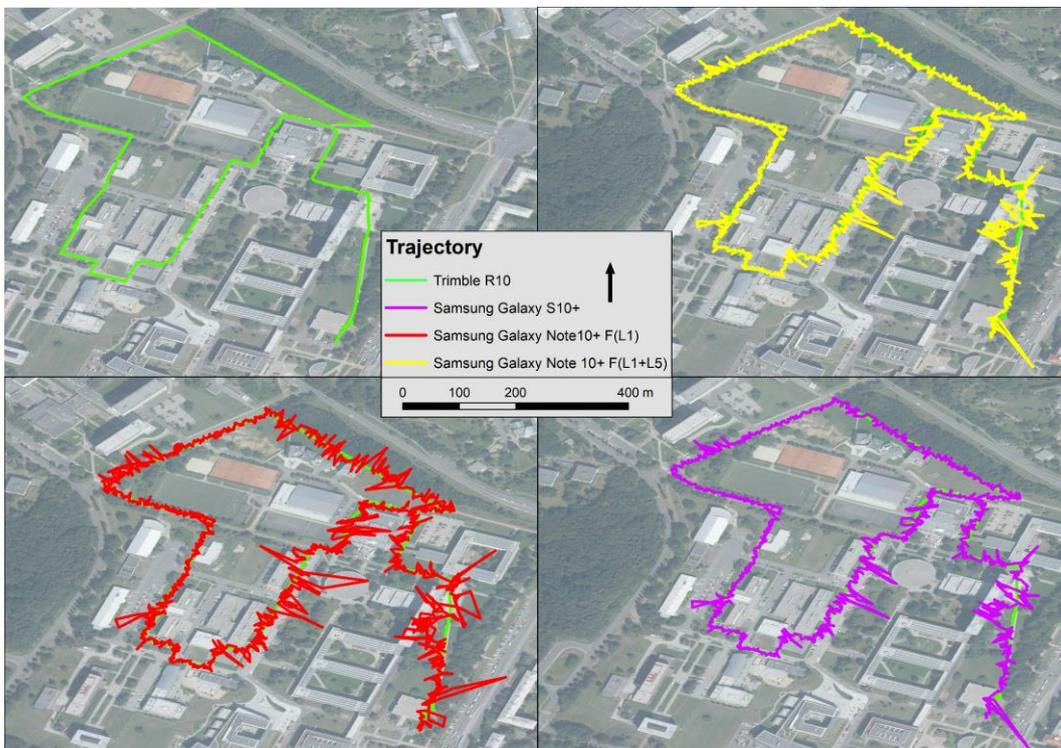
**Appendix D.** Estimated routes of tested devices using the Kinematic technique on November 16 (variants of post-processing with numbers 3 and 4, see [Table 5](#))
