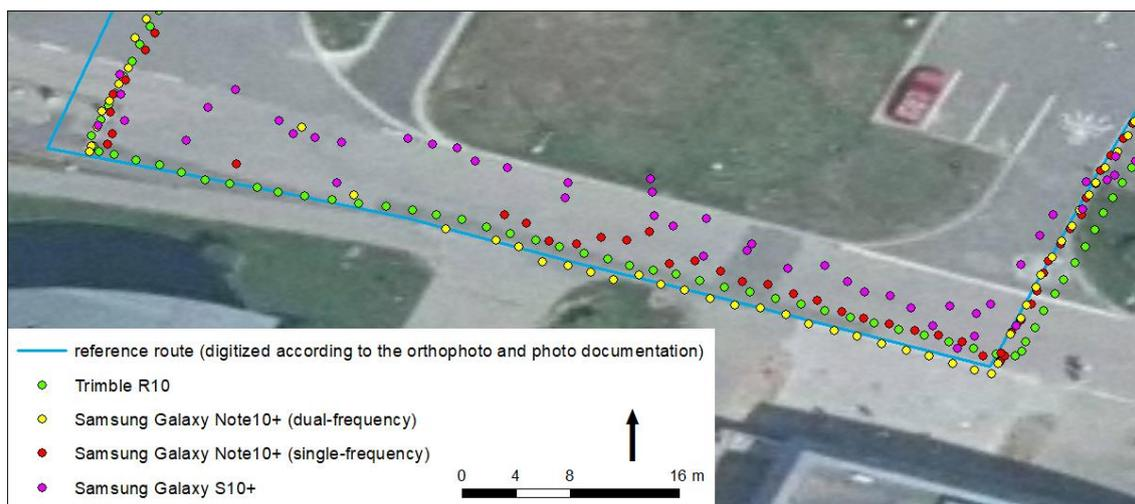
**Figure 3.** Illustration of individual positions of GNSS devices and the digitized reference line
