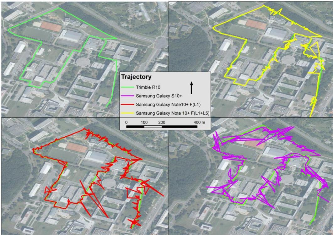
**Appendix C.** Estimated routes of tested devices using the DGNSS technique on November 16 (variants of post-processing with numbers 3 and 4, see [Table 5](#))
