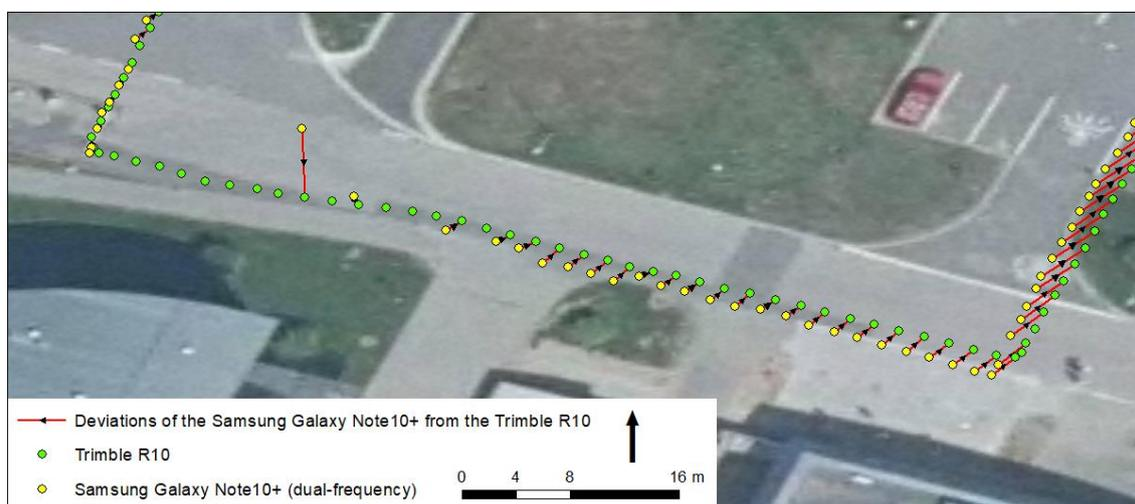
**Figure 4.** Illustration of the evaluation variant based on calculation of differences between the geodetic grade GNSS receiver and tested smartphones
