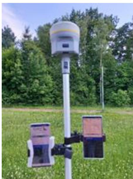
*Figure 2. Illustration of smartphone and reference receiver positions during data collection*
